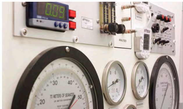
The operating control panel, including O 2 -CO 2 analyzer, depth and supply gauges, triple timers and a communicator.
