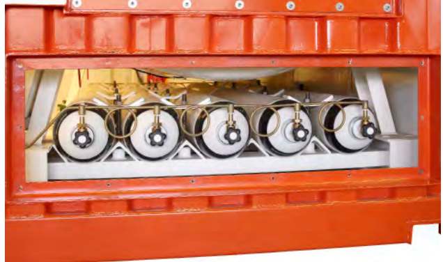
Gas cylinder location.
