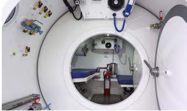
The entrance lock. In emergencies the entrance lock can be used as treatment chamber. The main chamber can be used for two patients laying down on the two stretchers, or three patients in sitting position
